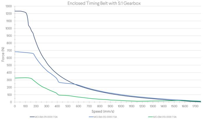
The above graph shows the driving force of the enclosed axis through the range of operational speeds when equipped with a 5:1 planetary reduction gearbox, MO-PT-001-0001. As with the earlier figure, the three different curves represent the actuator's performance with a gearbox and the three types of NEMA 34 motors offered by Vention: MO-SM-011-0000, MO-SM-012-0000, and MO-SM-013-0000, driven by MachineMotion 2.
